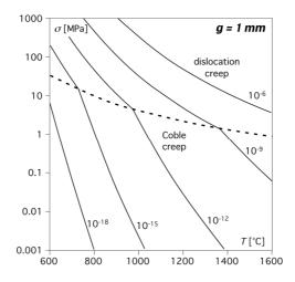
Deformation mechanism maps can be made for any pair of variables. We have already seen a standard combination of stress *vs* temperature (at a certain grain size). One can also make one for stress versus grain size at a certain temperature.
