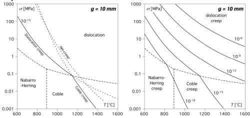
Let us draw the stress-strain rate curve for  $10^{-15}$  s<sup>-1</sup> in our deformation mechanism map:
